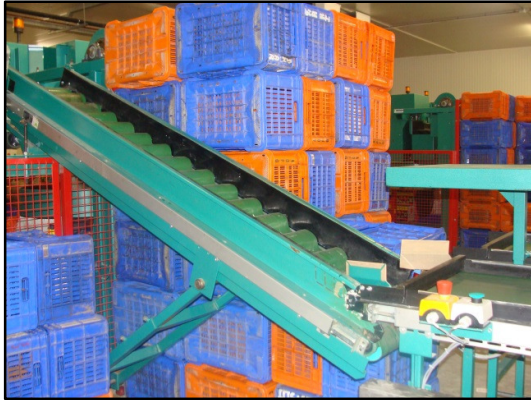
Figure 8: Conveyor belt of the sorting and grading equipment in the cold storage Source: OneWorld Foundation India 2013
